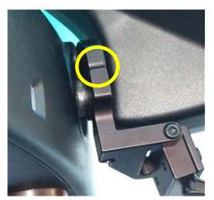
STEP 3 - When the pivot points are touching, tighten the clamp screw untill the Top and Mid Sections are slightly snug around the mirror stem. You should still be able to rotate the mount.
