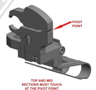
STEP 2 - BEFORE FULLY TIGHTENING THE CLAMP SCREW, MAKE SURE THE TOP AND MID SECTIONS ARE TOUCHING AT THE PIVOT POINT. If you can not get them to touch at the pivot point, you have an incompatible mirror type for this mount.
